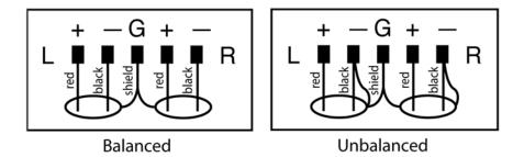
For unbalanced sources, connect the unbalanced source to one side of the balanced input and ground. The other input does not have to be grounded. Note, always use the same side of the balanced input for stereo.
