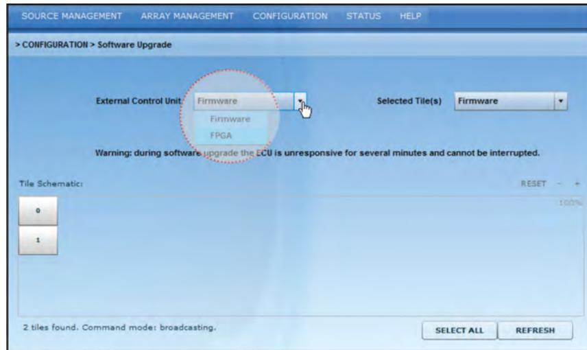
**Figure 3-36 Upgrading External Control Unit**
